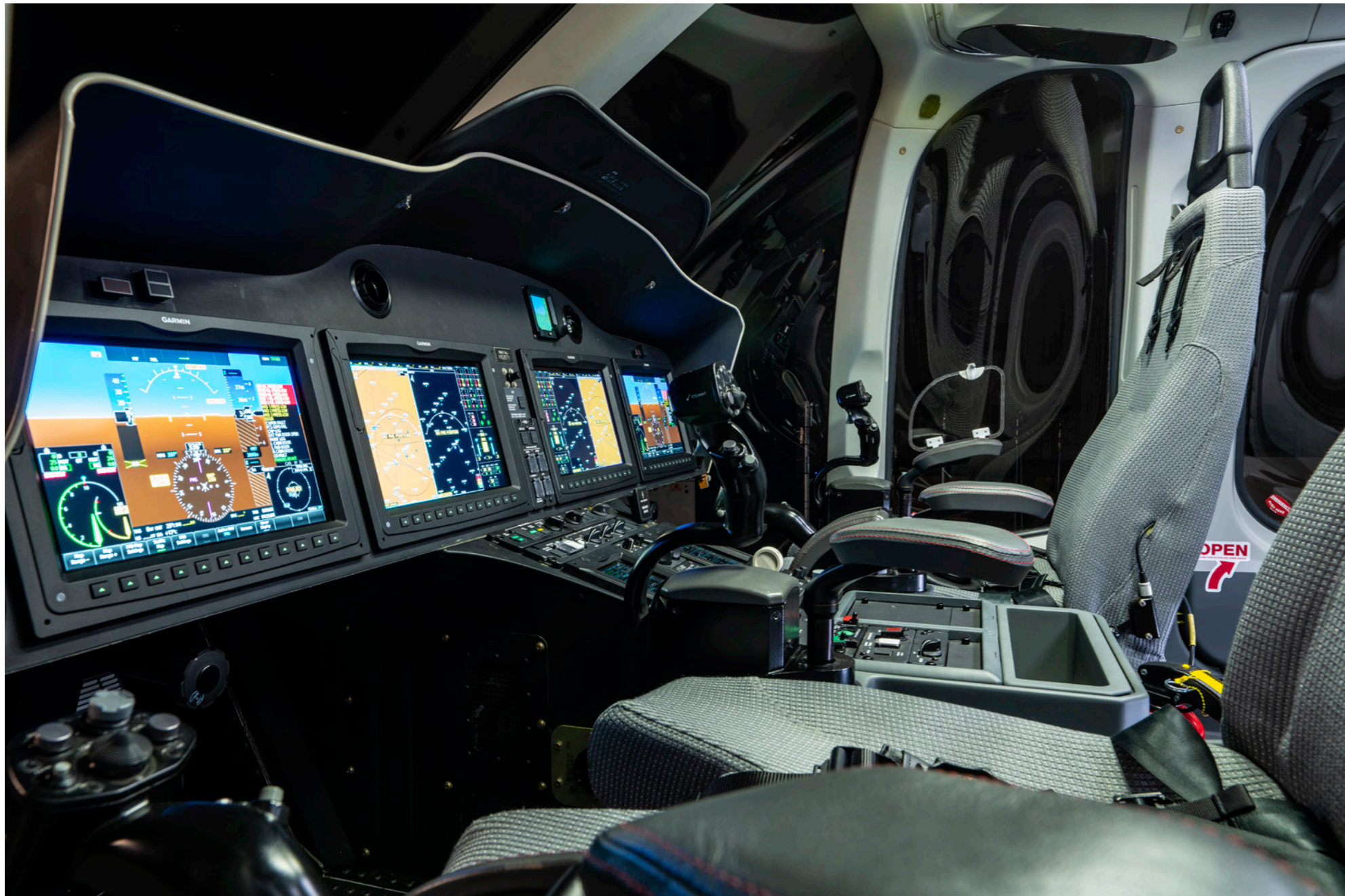
The Relentless is the first commercial helicopter to incorporate the Garmin 5000H, a touchscreen avionics suite. The Bell 525's standard configuration G5000H Flight Deck includes the HSVT (helicopter synthetic vision technology) that gives the pilots a 3D depiction of terrain, obstacles, traffic and more in any visibility condition
